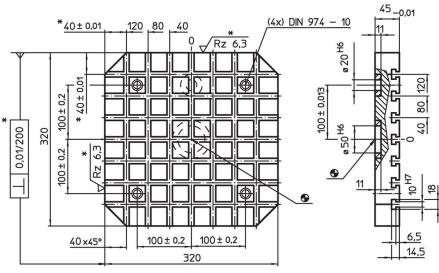
$^{\ast}$  These tolerances are valid only for optional exterior stop type. Slot spacing 40  $\pm0.01.$
